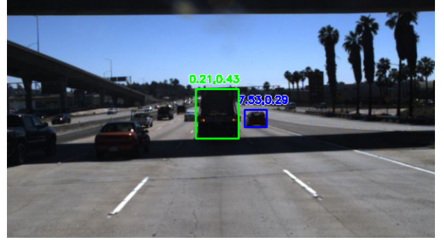
Fig. 1. Sample sequences from the TuSimple dataset at the last frame with their respective bounding box and velocity annotation in Z and X direction.
