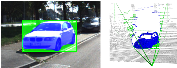
Fig. 3: For each pair, left: RGB input image with Mask R-CNN predicted box and highlighted pixels inside the mask. Right: LiDAR points in blue represent those inside the 2D mask, green those outside. Note that, while the image mask removes many outliers, many remain at the object boundaries and transparent surfaces.
